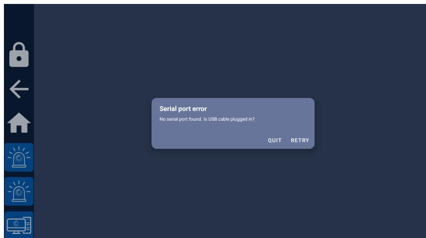
Figure 4: Error message when the MCS CAN Bridge USB cable is unplugged
